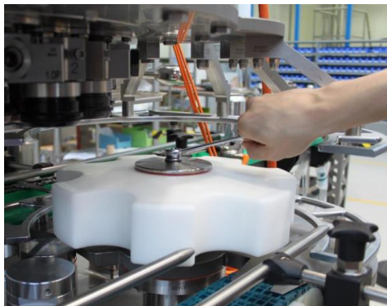
Fig. 17: Removing the discharge turret
